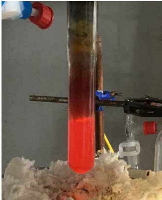
Molten FeCl 2 eutectic salt mixture
